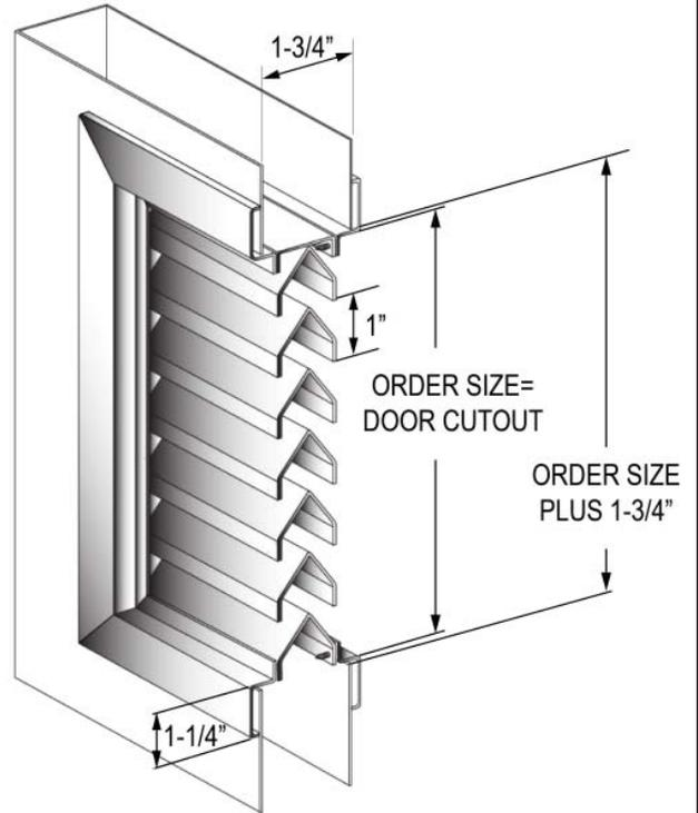
For use in Fire Rated door applications under positive and neutral pressure. Intertek testing certification in compliance to NFPA 252 (2000), UL 10C (2009), NFPA 252(2012) and CSI Code 089000 Louvers & Vents
