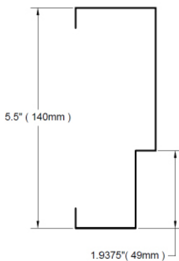
DRAWING PROFILE FOR SINGLE RABBET FRAME DEPTH 5.5"
