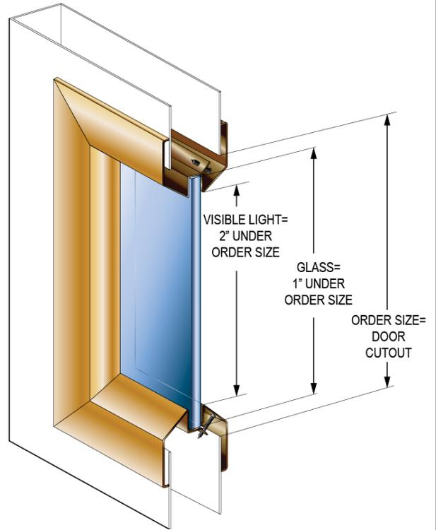
For use in Fire Rated door applications under positive and neutral pressure. Intertek testing certification in compliance to NFPA 252 (2000), UL 10C (2009), CAN/ULS104 (2010), NFPA (201) and CSI Code 0870 00
